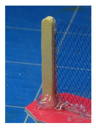
Once this is all set, you can build up the base with Polyfilla or similar, making it thicker as you come in from the edges of the base until the globs of glue are covered. Use a spare bit of plasticard or similar to spread and smooth the filler.
